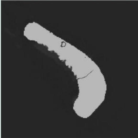
A standard X-ray CT image of a 3D-printed metal turbine blade shows beam hardening and streaking effects. Credit: Amir Ziabari/ORNL, U.S. Dept. of Energy
