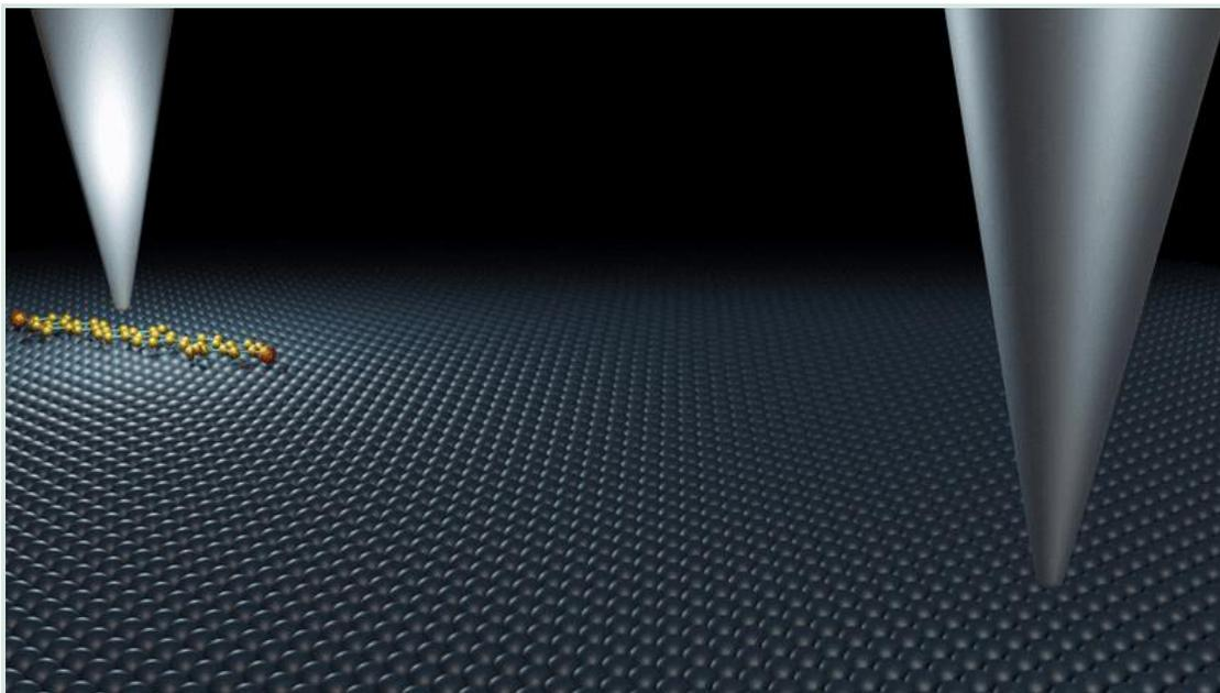
The animation depicts the controlled transport of a single molecule between two scanning tunneling microscope tips in an experiment at ORNL. Credit: Michelle Lehman/ORNL, U.S. Dept. of Energy
