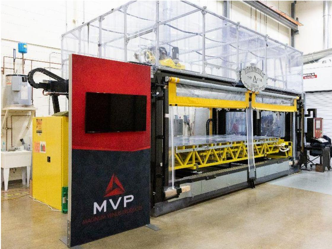
The Reactive Additive Manufacturing, or RAM, machine for large-scale thermoset printing supports two technologies licensed by MVP and developed in collaboration with ORNL. Credit: Carlos Jones/ORNL, U.S. Dept. of Energy
