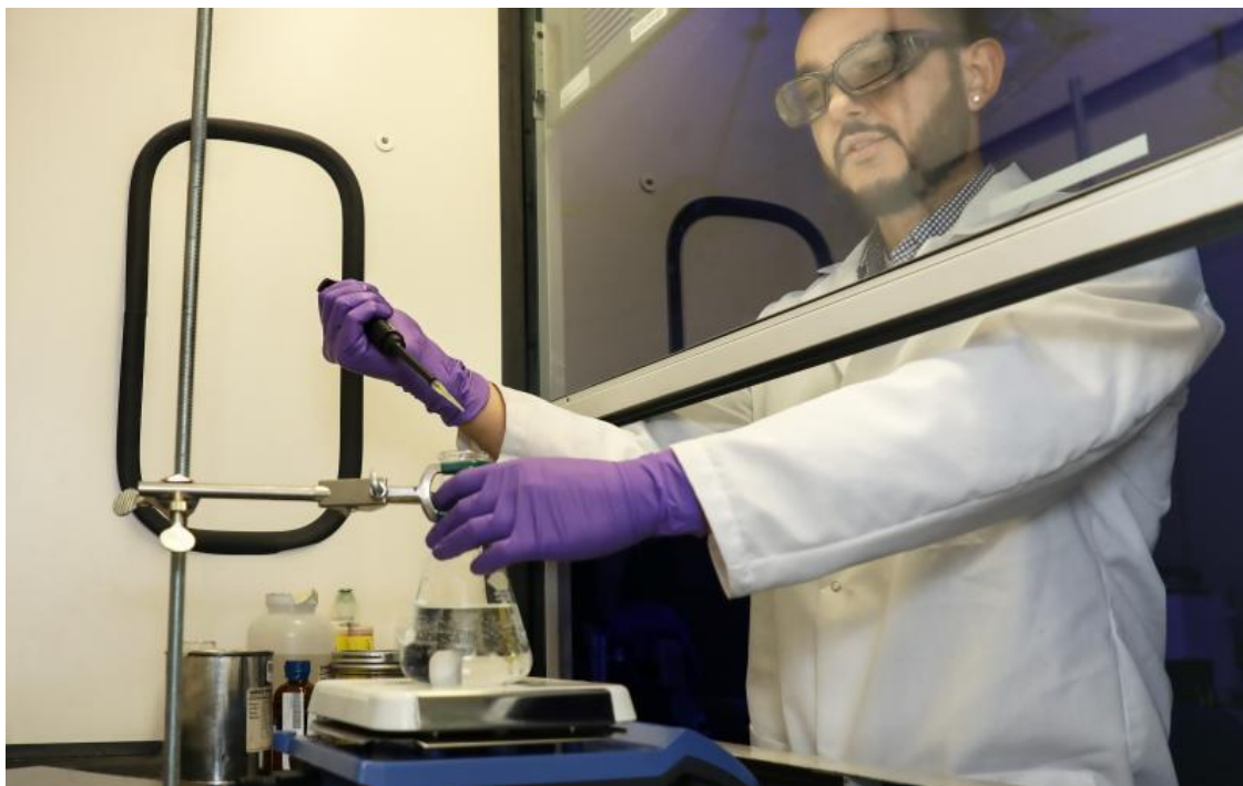
ORNL researcher Halil Tekinalp combines silanes and polylactic acid, or PLA, to create supertough renewable plastic. Credit: ORNL/U.S. Dept. of Energy
